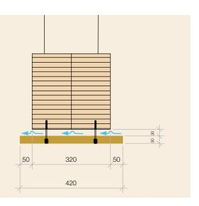
The anti-condensation panel can simply be exchanged. It protects the timber frame as a wear layer.
