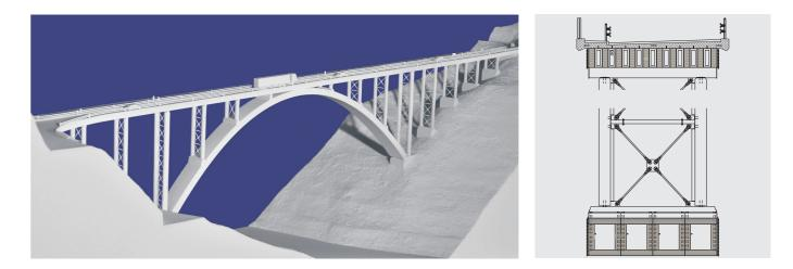
The 240-metrelong Vulpera wooden bridge with an arch span of 120 metres and a height of 70 metres.
