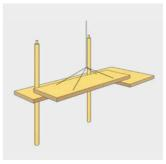
8×8 metre column grid With TS3, slabs bear load in two directions, spanning col-
